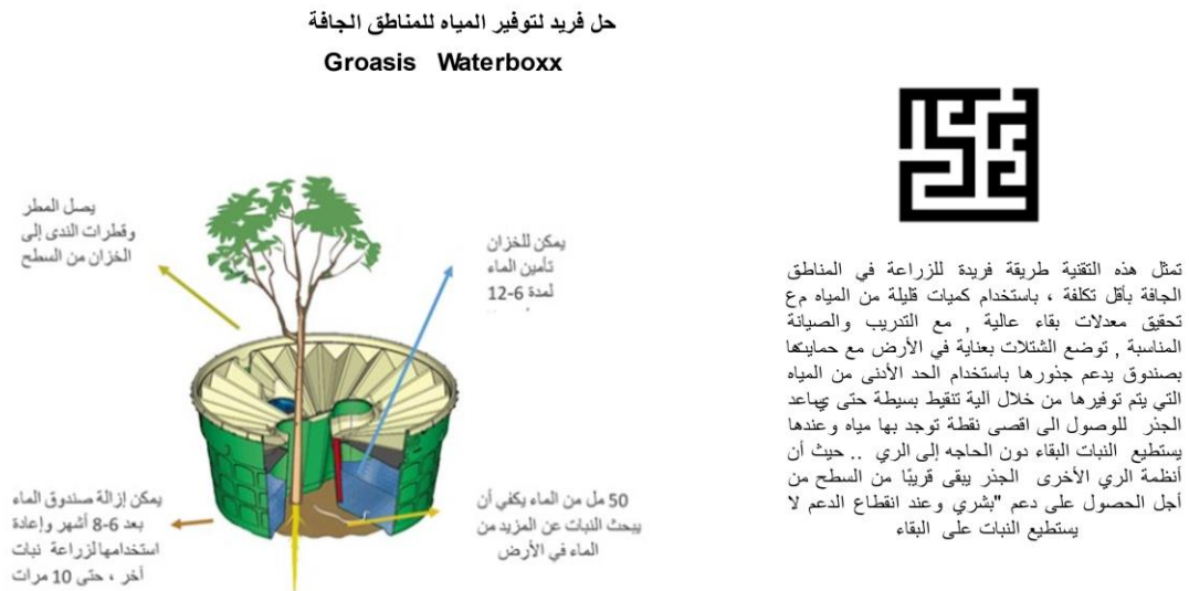
Figure 1: Illustration of Waterboxx functionality
